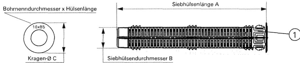
Ankerstangen M6, M8, M10, M12, M16
