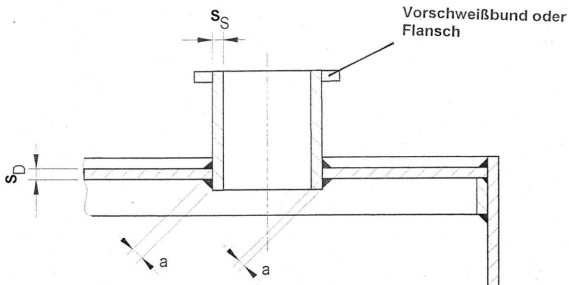
$$a \geq 0,7 s_{\min}(s_R, s_D) \quad (\text{WE, WZ})$$
