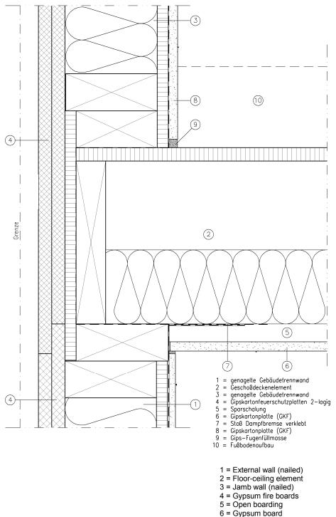
7 = Joint formation of the vapour barrier between external wall and ceiling
