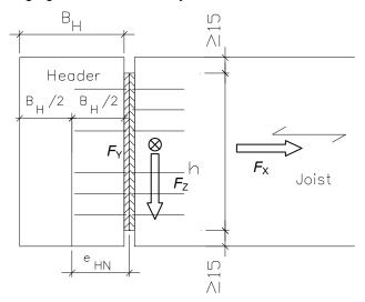
The ATF connectors are intended for use for connections subject to static or quasi static loading.
