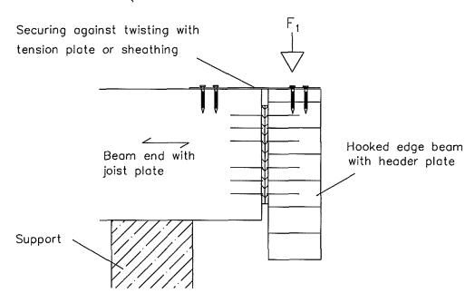
View of an edge beam — column connection with ATF connector (The connector is installed "normally")
