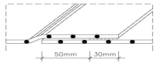
Lap joint without air-channel (single weld)
