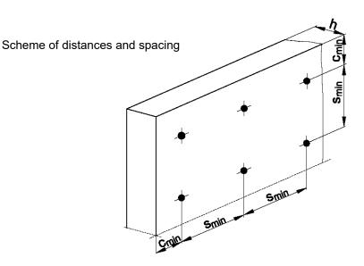
EJOT SDM-T plus, SDF-K plus and SDF-S plus
