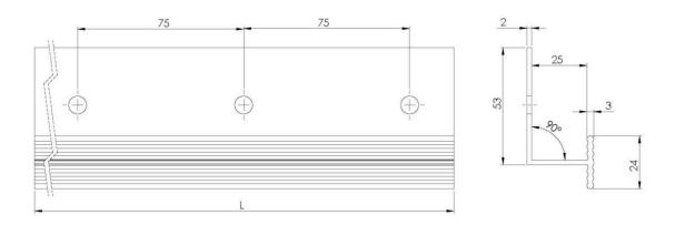
Vertical connection profile "Sto-Halteleiste PVC" (dimensions in millimetres)
