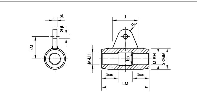
Minimum screw-in length of the tension rod = om - oj according to Annex B3 \* /.. alternative dimensions for a M10 tension rod connection
