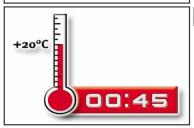
Temperature related curing time t<sub>cure</sub> (Annex B 5) must be observed. Do not move or load the fastener during curing time.
