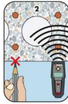
Mark the prestressing steel and locate the second prestressing steel
