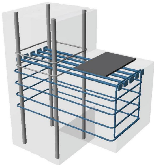
Corbel with Halfen Stud Connector type HSC-HD
