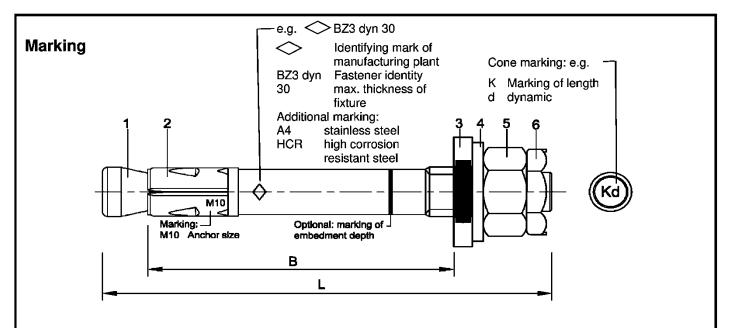
Usable length:  $B = h_{ef} + t_{fix}$
