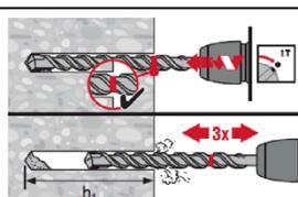
No cleaning is allowed in upward installation direction.
