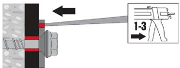
Fill the annular gap between screw and fixture with 1-3 strokes of a Hilti injection mortar HIT-HY ... or HIT-RE ....
